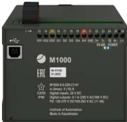
Single phase, 4 digital inputs, 2 digital outputs
